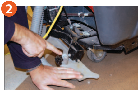
2 Lubricate pivot joints with light oil. Do not overuse.
