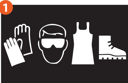
1 Before inspecting wet/acid batteries you are required to wear appropriate PPE (Nitrile chemical resistant gloves, goggles, apron, closed toe shoes)
