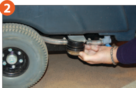
2 Inspect and clean solution filter.
