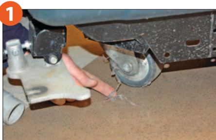
1 Inspect caster wheels and squeegee guide wheels for string/hair etc.
