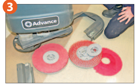
3 Remove pad holder and pad. Remove pad and rinse out. Hang to dry.
