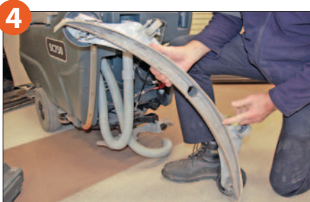
4 Remove and clean squeegee assembly. Check blades for wear or damage. Flip squeegee blades if required.
