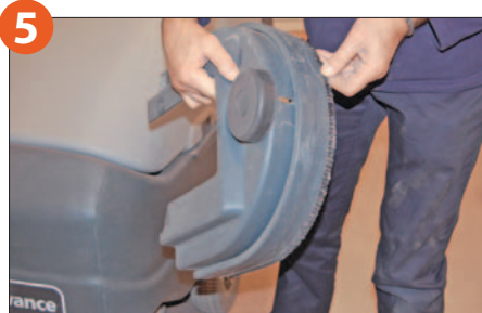
5 Check bumper wheels and brush skirts for damage.
